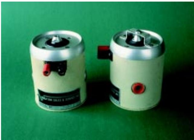
Figure 8. Mechanical configurations for traditional coil impedance tests. The unit on the left is unrestrained; the shaker on the right has its table motion “blocked” by a bracket.
