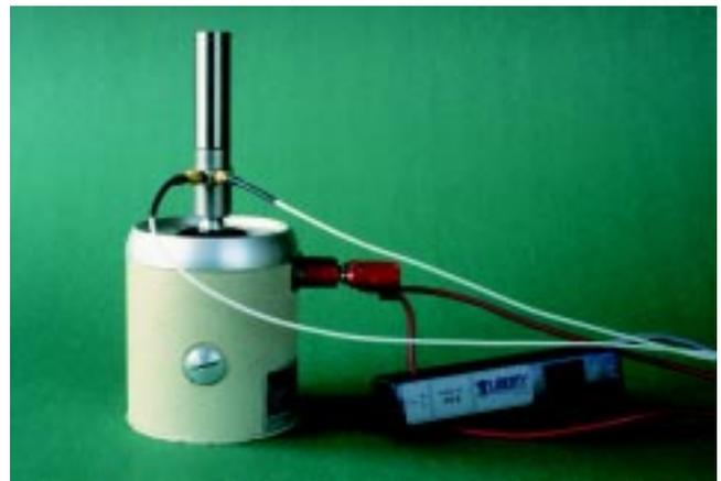
Figure 11. Experimental arrangement used to illustrate force/motion/voltage/current relationships. The current driving the shaker is monitored by a clamp-on instrument-grade current transformer. An ICP impedance-head measures the force delivered by the shaker and the motion of its table. A 76.97 gram stainless-steel cylinder is fitted as a test mass.
