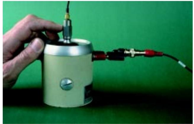
Figure 2. "Pluck" testing a shaker. The finger depresses the table against its limit stop, then releases it abruptly. The transient voltage generated by the shaker coil is measured with a high impedance instrument.
