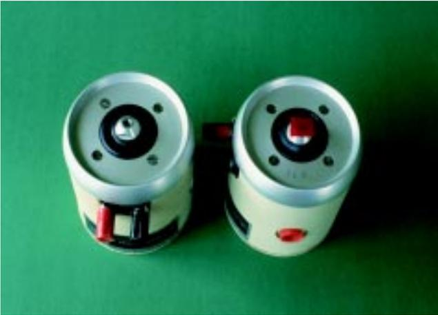
Figure 5. An unanticipated discovery; this shaker's damping is predominated by internal aerodynamic effects. The "pluck" test was conducted on a shaker with an open mounting hole (no stud) and on a unit with the hole blocked by plastic tape.
