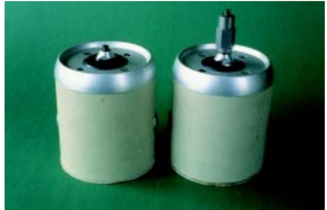
Figure 1. Two small electrodynamic shakers illustrate the mass loading used in "pluck" tests. The unit on the left has an (essentially) bare table; only a 0.72 gram beryllium-copper 10-32 UNF mounting stud is installed. A 23.61 gram accelerometer is fitted to the unit on the right.
